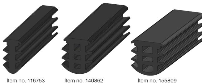
The milled groove of the optical guidance system must be sealed against environmental conditions. A simple and low-cost solution is to use the halogen-free GIFAS system profile made of EPDM. This is inserted in the slot. It is self-locking and available in three different widths. A stable and smooth slot with slot widths of 6 -15 mm is the prerequisite for use.
